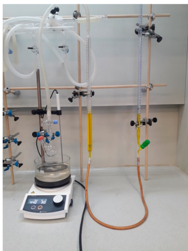
Figure 3. Experimental setup for the measurement of the molecular hydrogen evolved.
