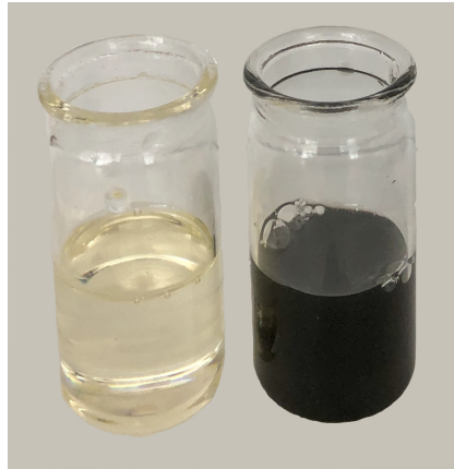
Figure 9 Therminol 66 (left) and Therminol 66 with carbon black nanoparticles (right).
