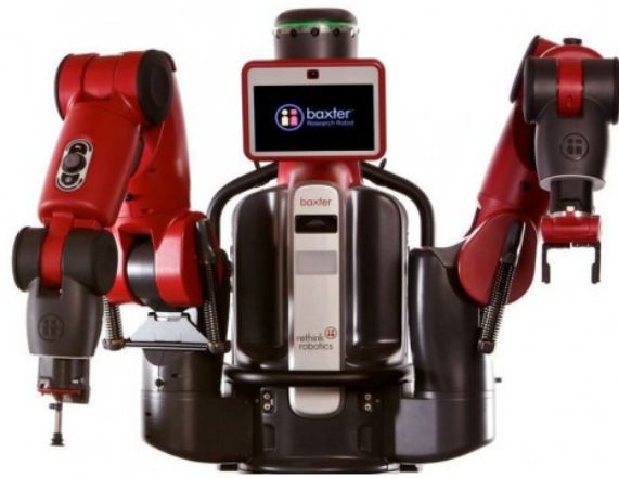
Figure 2.1: BAXTER is one of the most popular robots used by the research community. This is a representative image of BAXTER, and the grippers were custom made for the modified Picking and stowing task.
