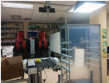
Figure 2.2: Front view of the setup. The small black box hanging above is the KINECT. The shelf can be seen on the right side of the image.
