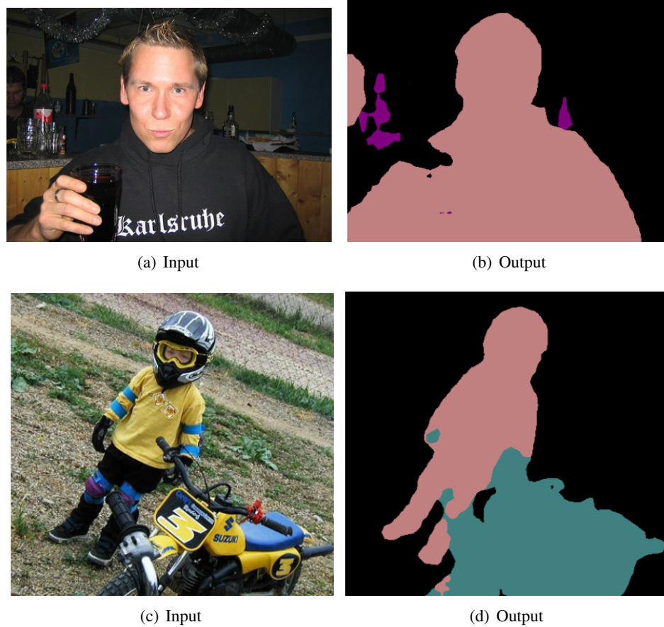
Figure 3.8: RESNET trial on VOC2012 segmentation test dataset. It should be noted that the different classes are denoted by different colors.
