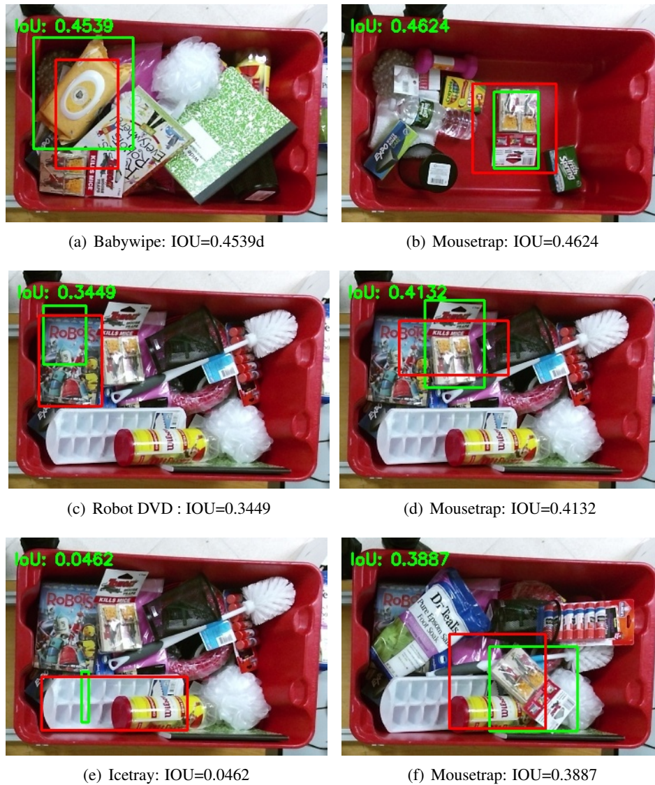
Figure 5.7: YOLO produces detection result which is mostly unreliable for object detection. In some cases, as shown above, it detects the wrong object and sometimes outside the coordinates of the frames. It is to be noted that this result has been produced after 57000 iterations.
