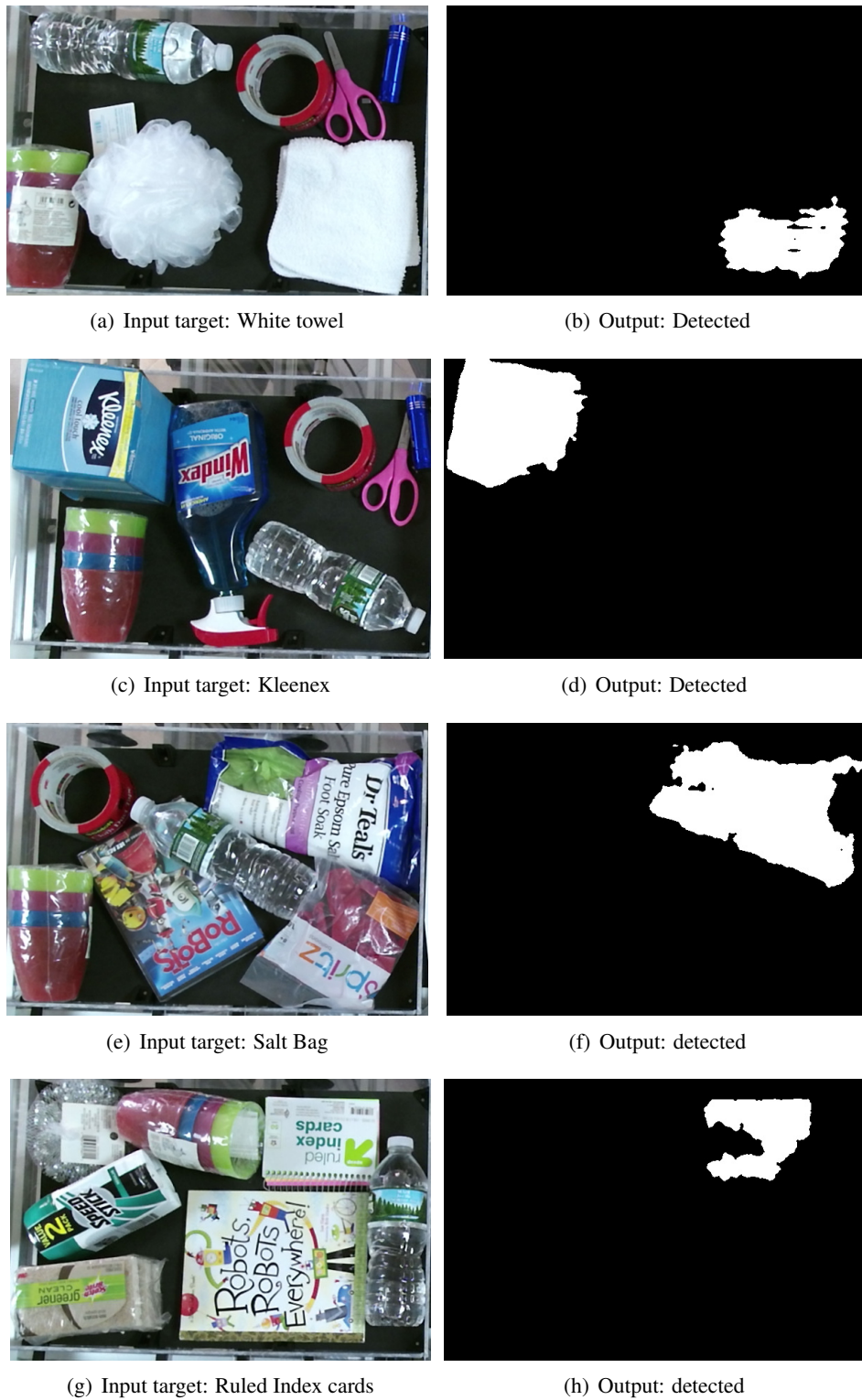
Figure 5.5: Accurate depiction of the target items through semantic segmentation (RESNET). Total iterations in this case is 4500. This seems to be a concrete option for object recognition for picking task.
