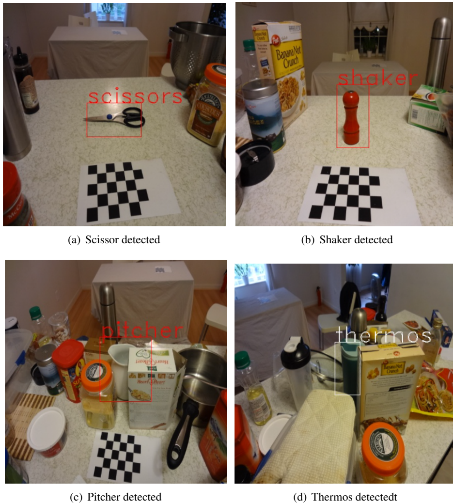
Figure 3.3: YOLO trial on CMU kitchen dataset after 8000 iterations. This is a sample run on cluttered dataset example. This is to check the validity before the original test on AMAZON dataset.
