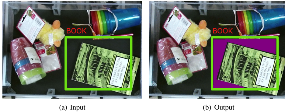
Figure 5.1: YOLO output of book. Although detection is done with a high accuracy, there is a lot of redundant space inside the ROI (Region of Interest). The purple region denotes the redundant space and any wrong item, if present might be picked up by the gripper due to detection of point-clouds not belonging to the item in the ROI.
