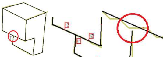
Fig. 3. T-junction (left) may either split the second line (centre), or ensure that the first line touches the second (right)
