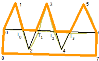
Figure 10. Two segments of the same line, delimited by pairs of T-junctions, belong to the perimeter
