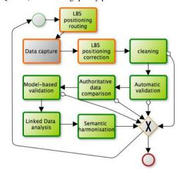
Figure 1: Typical workflow for quality assessment of crowd-sourced data before and after data capture (BPMN diagram)
