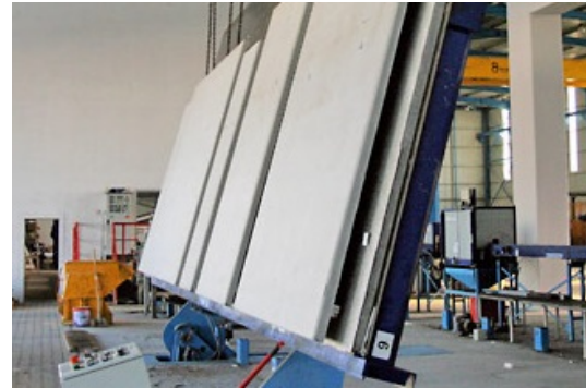
Figura 4.32: Desmoldeo muro doble. Ref. VOLLERT
