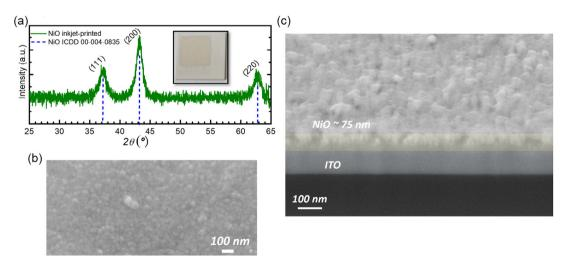
Figure 1. a) XRD pattern on IJP NiO showing characteristic peaks of cubic phase NiO. Inset shows the picture of a transparent IJP NiO film on glass substrate; b) top-view SEM image of IJP NiO; c) Cross section of the IJP NiO thin film by the FIB-assisted FESEM technique. The layers have an ITO bottom electrode thickness of 100 and 75 nm of NiO.
