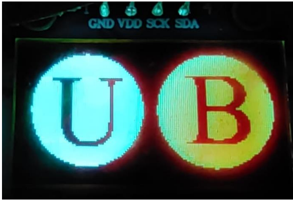
Figure S5: Optical photo of the CsPbI 3 perovskite CCL excited by the back blue InGaN-based micro-LED display. ATR characterization of inkjet-printed CsPbI 3 with expected signals for this LHP.
