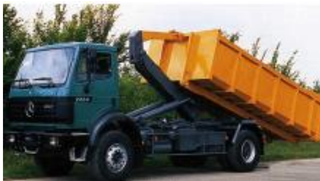
Imagen 49: Camión Hooklift. Fuente: (UN-HABITAT, Collection of Municipal Solid Waste in Developing Countries, 2010)
