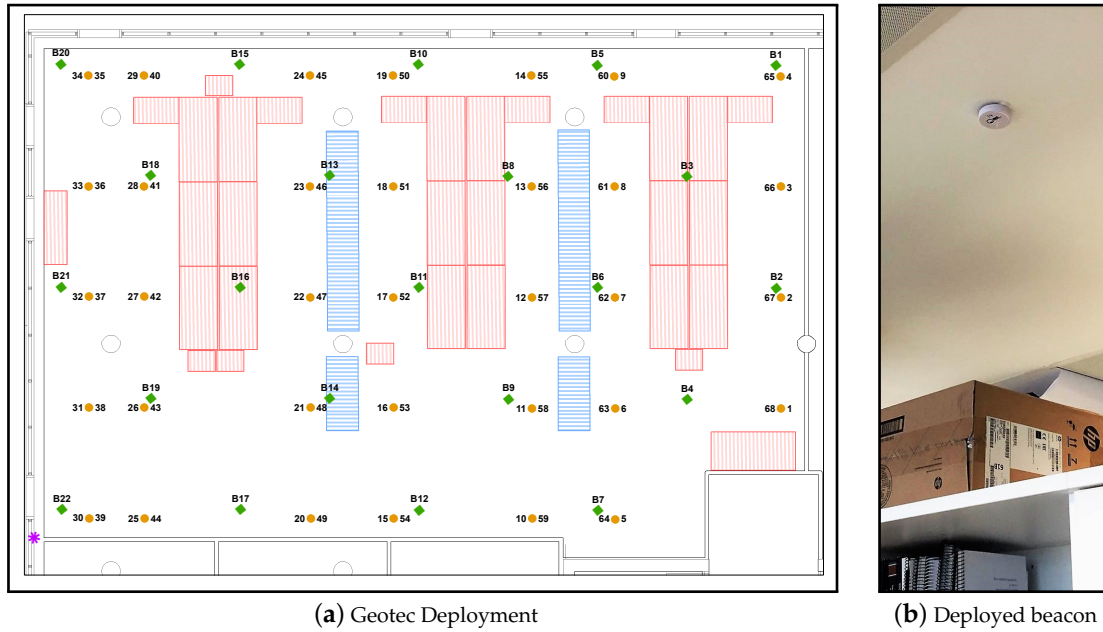
Figure 3. Geotec office zone. In (a), green diamonds, orange circles and the magenta asterisk represent the position of beacons, collection locations and the local coordinates origin, respectively. The blue horizontal-lines-filled rectangles represent tall furniture that create NLOS situations. In (b), a shot to show how beacons were deployed in the ceiling tiles.
