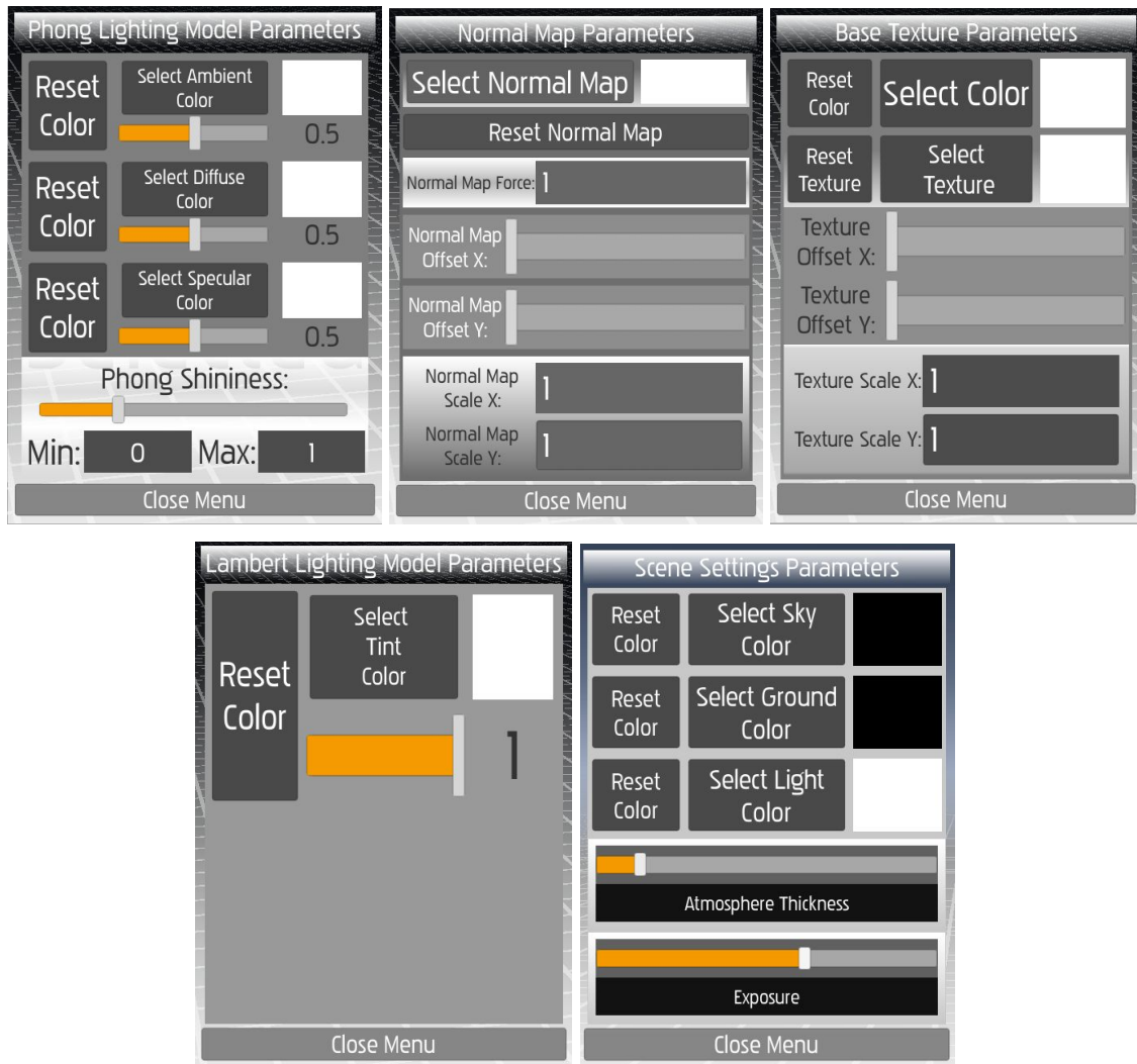
Figure 13. Final design of all the secondary Menus. From left to Right, from top to bottom: Phong Lighting Parameters Menu, Normal Map Parameters Menu, Base Texture Parameters Menu, Lambert Lighting Parameters Menu, and Scene Settings Parameters Menu.
