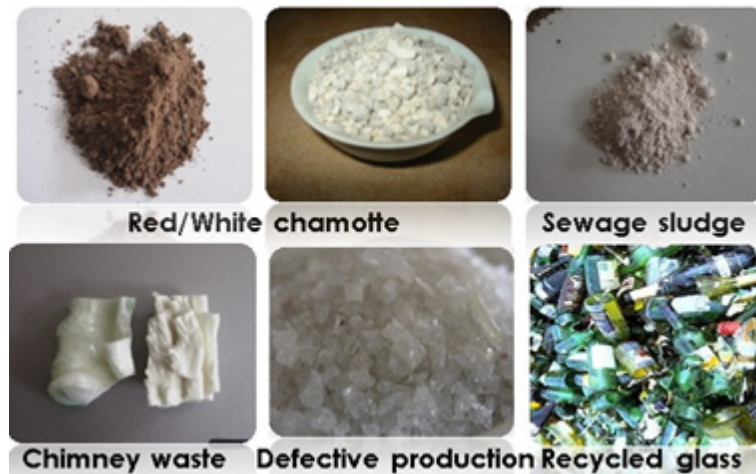
Fig. 1. Recycled materials applied in the preparation of the eco-ceramic and glass ceramic bodies (pastes).
