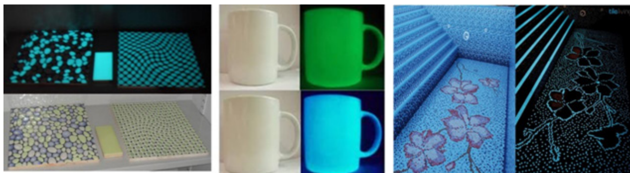
Fig. 13. Some applications of phosphorescent ceramics.
