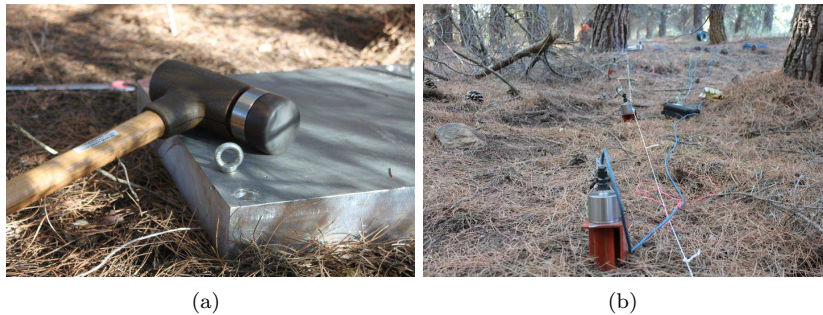
Figure 5: SASW test: (a) impact hammer and aluminium foundation; (b) accelerometers setup.
