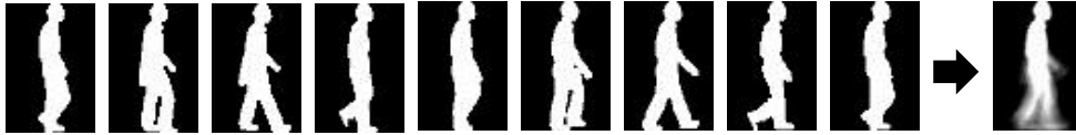
Fig. 2 Gait sequence through a series of key silhouettes, and the resulting Gait Energy Image (GEI).
