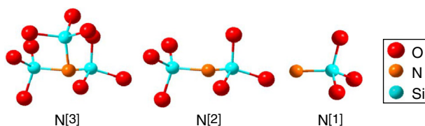
Fig. 5 – Possible links of the nitrogen atoms in a silicon oxynitride network [29].
