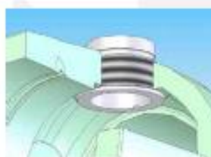
Flat surface formed in the vessel shell - reduces center lining
