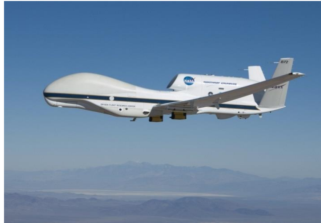
Figure 3: Global Hawk, NASA's unmanned aircraft system for high-altitude, long-duration Earth science missions [5].
