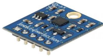
Figure 5: 3-Axis Digital Compass HMC5883L used in AR.Drone 2.0 [43]
