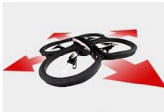
Figure 21: Pitch and roll movements [3].
