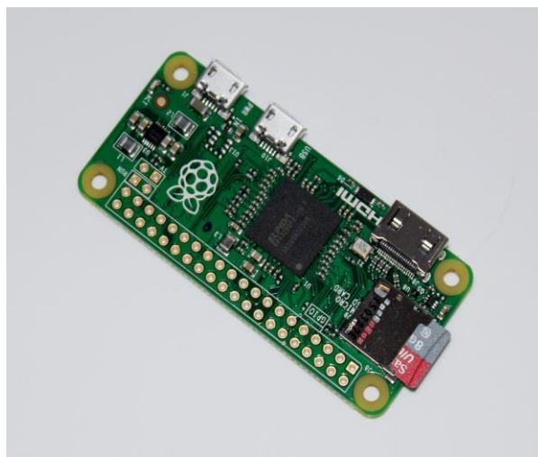
Figure 26: Raspberry Pi Zero. Its size is ideal for this project because it can be installed inside the hull of the AR.Drone 2.0 [52].
