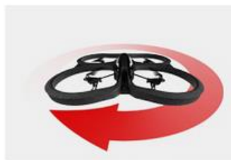
Figure 22: Rotation movement about its vertical axis [3].
