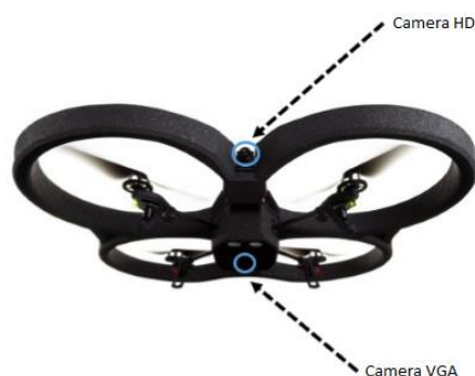
Figure 38: Front and bottom cameras in AR.Drone 2.0, cameras used to read QR codes and observe the environment.
