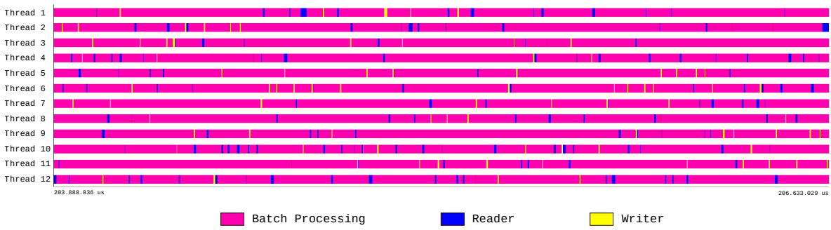
Fig. 8: Trace (fragment) illustrating the pipelined execution of Work-flow 1 with 12 threads/cores. Each horizontal bar shows the type of activity performed by one of the threads at a given time. The execution yields an interleaved execution with, e.g., I/O from/to disk proceeding in parallel with the batch processing. The trace shows there are at most one reader and one writer at any time.
