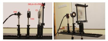
Fig. 7. Experimental micro-Köhler projection system shown from two different directions.
