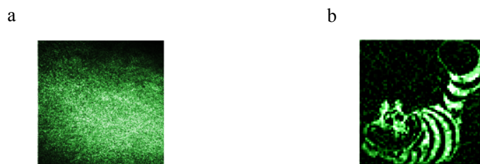
Fig. 2. Seeing through scattering media with a single-pixel camera. (a) The Cheshire Cat is placed in front of a scattering layer that completely hides it. We show the image of the object as seen by a charge-coupled-device camera (Stingray-F-145 with square pixel size of 6.45 \times 6.45 \mu\text{m}^2 ). The image contains not information at all on the shape of the object. (b) Image of the retrieved object from the photodetected values recorded by the photodiode. The good quality of the reconstructed image confirms that disorder-assisted imaging can indeed recover fine details of the object even though a sensor without spatial resolution is used.
