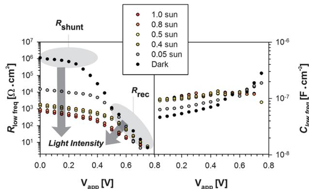
**Fig. 4** Analysis of the low frequency response obtained using impedance spectroscopy for a device based on the PTB7:PC<sub>60</sub>BM system (Device 5) measured under different light intensity conditions. The shunt resistance dramatically decreases with increasing light intensity and recombination kinetics is enhanced. Under high light intensity conditions leakage current is high, no carriers are stored carriers, and no chemical capacitance is observed.
