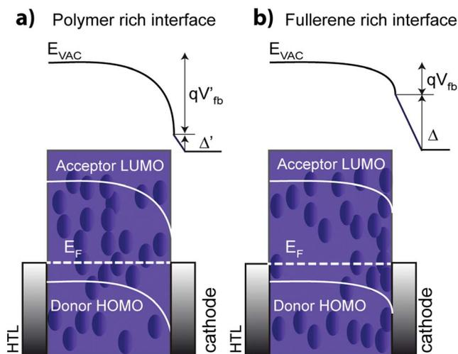
**Fig. 6** Schematic representation of dipole layer formation and band bending contribution on the active layer/cathode interface equilibration. (a) Interfaces with high polymer coverage show large dipoles and low band bending contribution and (b) fullerenes covering the contact display small dipoles and large contribution from band bending.
