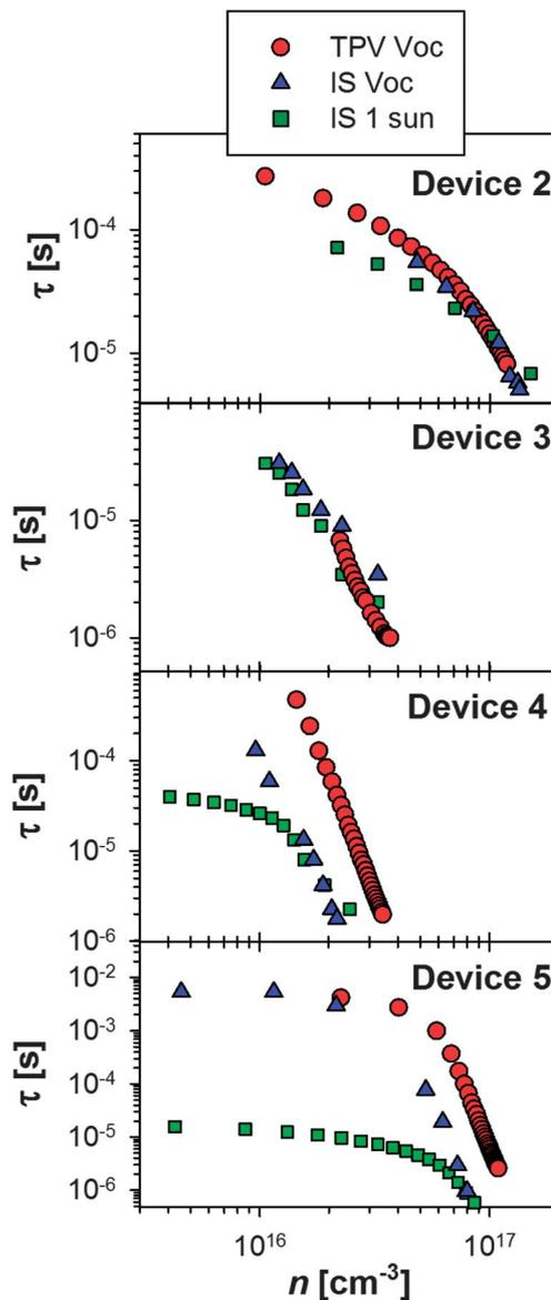
**Fig. 5** Charge carrier lifetimes of representative devices based on either P3HT:PC<sub>60</sub>BM or PTB7 at different carrier densities. TPV and IS measurements were performed under open circuit conditions and different illumination ( $V_{oc}$ ) or under constant illumination.
