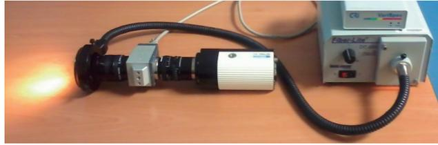
Fig. 1. Multispectral image acquisition system.
