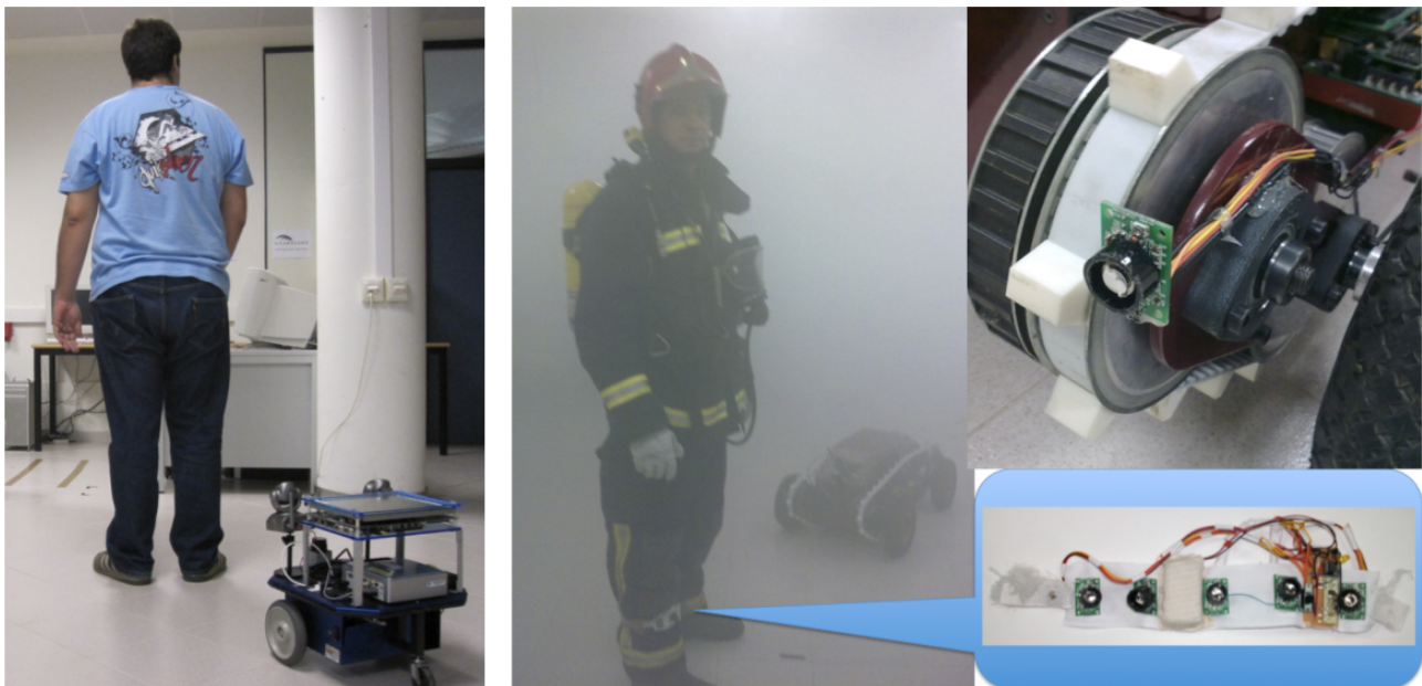
Figure 1. Robot following a human using computer vision (left). Robot following a firefighter using ultrasound and radio sensors. An ultrasound ring transmitter is attached to the firefighter's leg. The robot can follow the firefighter using the received signals (right).
