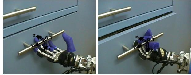
Fig. 15 The Armar-III humanoid robot pulling open the door of the dishwasher.
