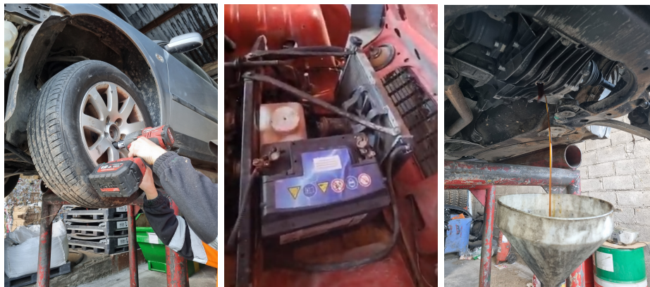
(a) Process of removing the wheels (b) Process of removing the battery (c) Process of removing the motor oil
