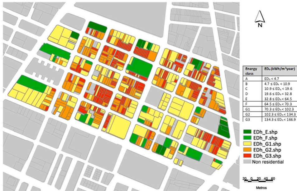
Fig. 3. Energy map for the ED h of the buildings in the neighbourhood.
