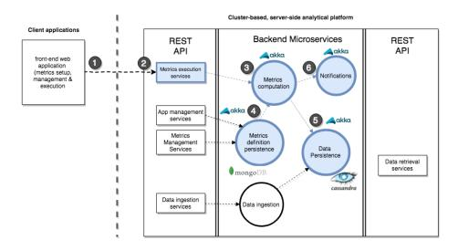
Figure 8. Coloured in blue microservices involved in the metric computation phase.
