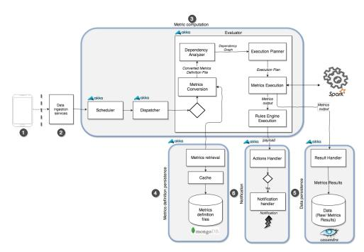
Figure 9. Data flow and involved micro-services in the Metrics computation phase
