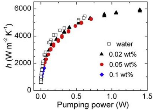
Heat transfer comparison at fixed pumping power for MWCNT nanofluids
