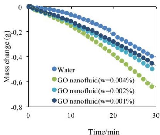
This figure shows time variations of the reduced mass of the GO nanofluid at different nanoparticle concentrations compared to that of water exposed to the light intensity of 3.5 Suns
