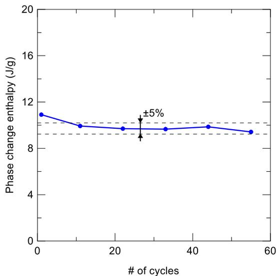
Evolution of phase change enthalpy with thermal cycling for a solar salt based nanofluid with 10 wt.% of Al-Cu nePCM to corroborate thermal stability.
