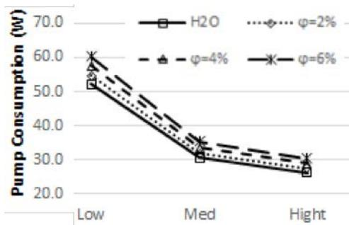
Pumping consumption for different nanoparticles concentrations.
