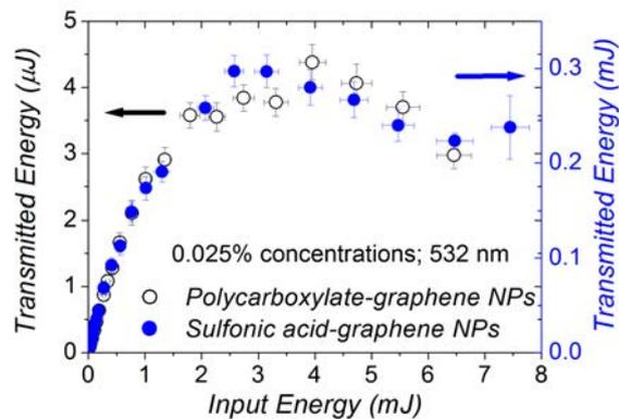
Optical limiting is evidenced also considering the dependence of Transmitted Vs Input energy. The plots refer to differently-functionalized graphene nanoplatelets under 532 nm wavelength [2].
