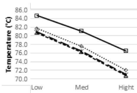
Outlet radiator temperature for different nanoparticles concentrations.
