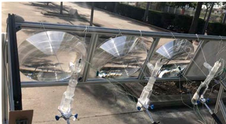
DASC system with concentration and solar tracking system for different fluids at a time
