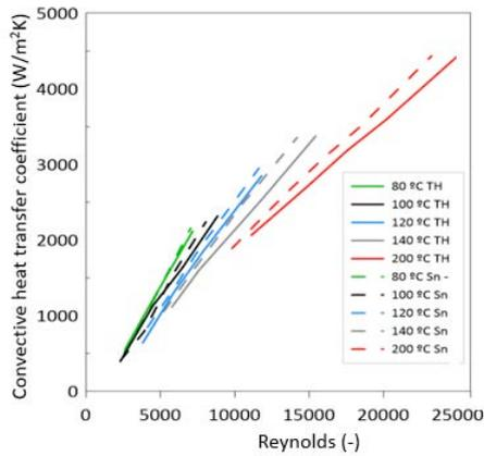
Heat transfer coefficient versus  $Re$  at different temperatures (from 80° to 200°C) for base fluid (Therminol 66, TH) and nanofluid (1 wt.% tin nanoparticles, Sn)
