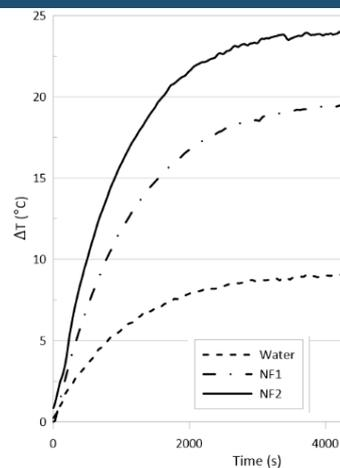
DASC system with no concentration and controlled room temperature and solar simulator (left) and increase of measured fluid temperature of water and water based nanofluids in two concentrations (right)
