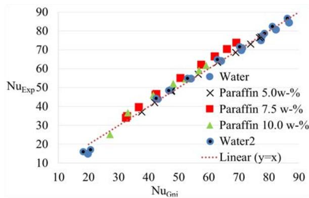
The convective heat transfer compared to the Gnielinski correlation (transition and turbulent regimes,  $Re > 3000$ ) for phase changing paraffin nanofluids. [Sep1]
