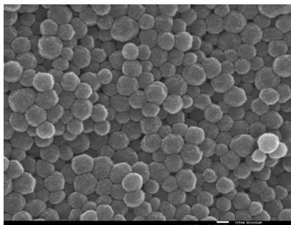
(SEM) image of melanin obtained from *Sepia officinalis* after isolation according to the method of the present invention, magnified 50 000 X.
