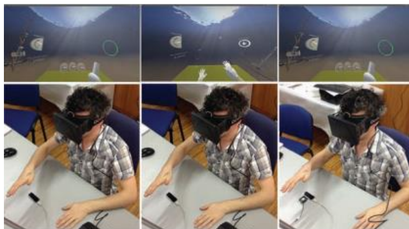
Figure 7. Multiple LM control, HMD and LM(left), with user in VR(middle) and with airflow-based haptic feedback(right).
