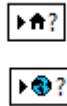
Figure 4.1.1.14: Up (element to create a local variable) and down (element to create a global variable)
