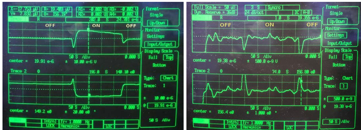
Figure 2. EC effect on thermal 3 \omega signals in TiO 2 Nf: (a) sdPP and (b) isdPP
