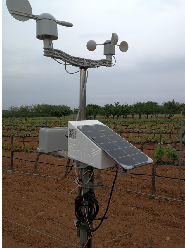
Figure 3.3.: Fully assembled and deployed SEnviro node.
