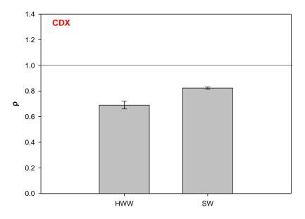
**Figure 4.** Treatment of representative antibiotics by ultrasound in distilled water (DW), hospital wastewater (HWW) and seawater (SW). (A) CLX antibiotic. (B) CDX antibiotic. Ultrasonic conditions as indicated in **Fig. 1**.
