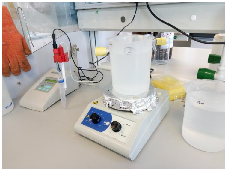
Picture 1. Example of one of the solutions prepared to carry out the dissolution stability test on continuous stirring.
