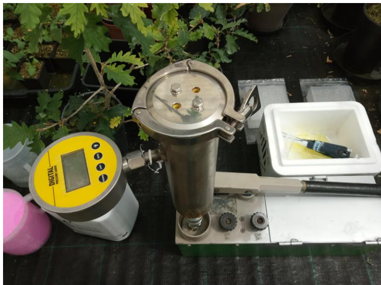
Picture 6. Pressure chamber similar to Scholander's chamber used to extract sap to carry out the tests.
