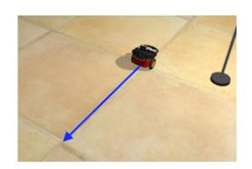
According to the specifications, the diameter of the wheels of the Pioneer 3DX robot is 195.3 mm.
