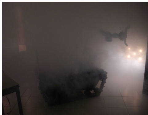
Figure 6. Testing Visual Pose method with high density smoke
