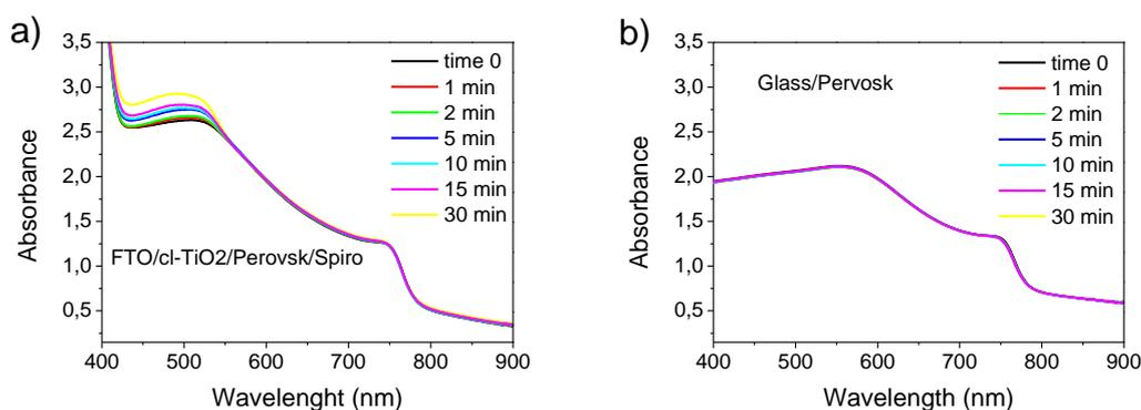
**Fig. 1.:** a) UV-VIS absorption evolution of a complete device without the top metal contact (FTO/cl-TiO<sub>2</sub>/PS/Spiro) and b) of a PS film on glass, at different illumination intervals under the solar simulator.
