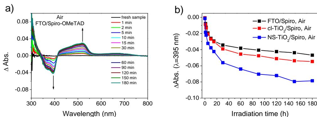
**Fig. 3.:** a) Evolution of the UV-VIS absorption signals of a Spiro film deposited by spin-coating on a FTO substrate. b) Evolution of the absorbance ( $\lambda_{\max} = 395$  nm) under 1 sun of a Spiro film deposited on FTO (black), cl-TiO<sub>2</sub> (red) and NS-TiO<sub>2</sub> (blue) in air, respectively.
