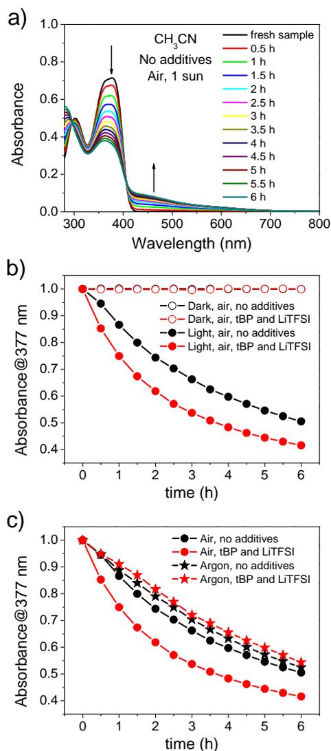
**Fig. 2.:** a) UV-VIS absorption evolution of a Spiro solution ( $10^{-5}$  M) in acetonitrile illuminated under 1 sun in air. b) Evolution of the absorbance ( $\lambda_{\text{max}} = 377$  nm) in the dark (hollow) and under 1 sun (solid) with the absence (black) or presence (red) of additives in air. c) Evolution of the absorbance ( $\lambda_{\text{max}} = 377$  nm) under 1 sun with the absence (black) or presence (red) of additives in air (circle) and in Argon (star).
