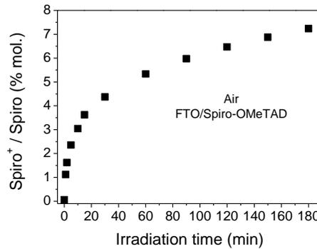
**Fig. 4.:** estimation of the Spiro<sup>+</sup>/Spiro molar ratio of a FTO/Spiro film under 1 sun at different illumination times.
