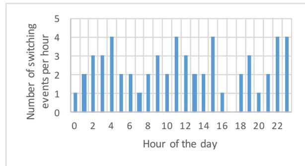
*Figure 2. The frequency of switching (on and off) of a fridge on one particular day. It can be seen that the frequency changes throughout the day with a noticeable reduction at 5 p.m. (17) when the fridge door was being frequently opened*
