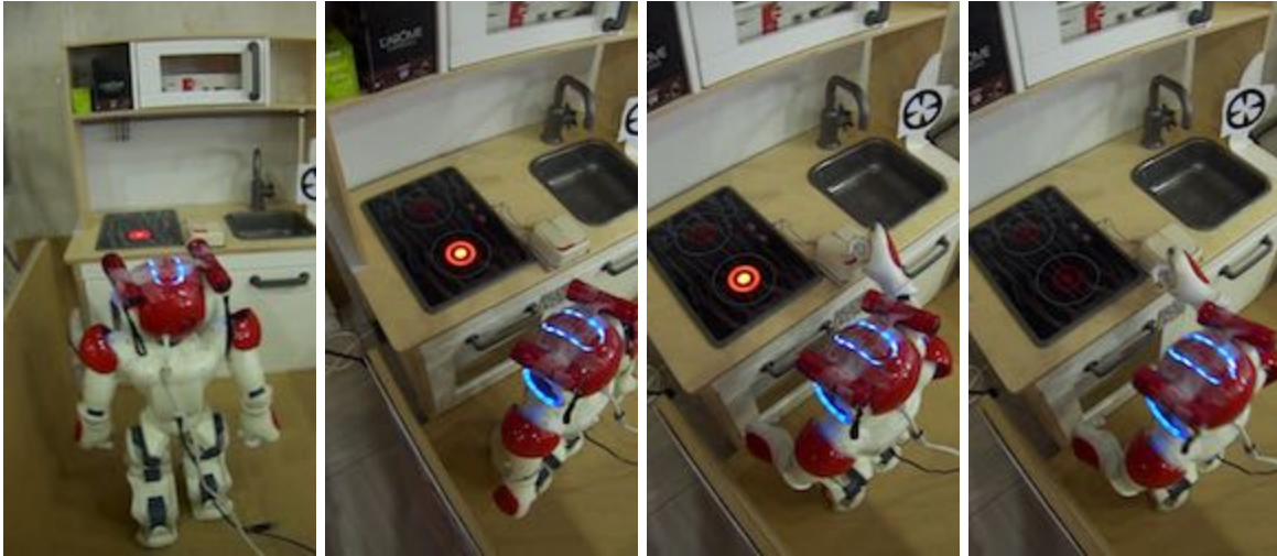
Fig. 4. Snapshots of the first test by the UPC team: the robot approaches the kitchen (1), detects the lit fire (2), moves its end-effector towards the button (3), and switches it off (4).
