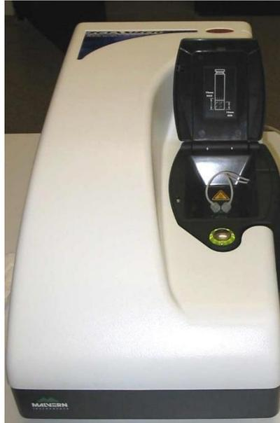
*Figura 5. Zetasizer Nano ZS (Malvern Instruments 226 Ltd., UK).*
