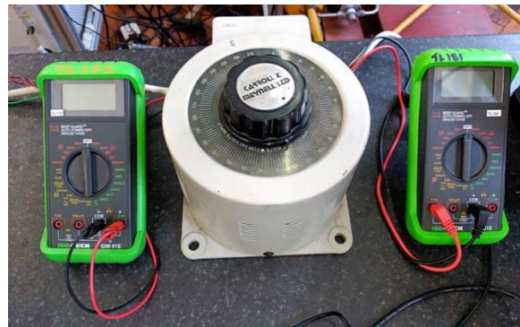
Figure 13: Power Supply to Cartridge Heaters
