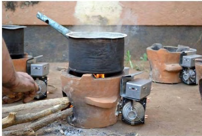
Figure 2: Completed Generator stove
