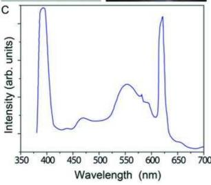
Figure 6. A) A photograph of MOF-PEMA-3.5 hybrid materials. B) The hybrids bright white light emission under excitation by a 395 nm GaN chip and C) the corresponding LED electroluminescent spectrum. Reproduced with permission. [76] Copyright 2014, Royal Society of Chemistry.
