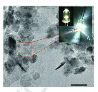
Figure 5. A) Photographs of the as-fabricated WLED using boehmite-based organic-inorganic hybrid nanoparticles operating at 3.0V. B) Representative TEM image of the boehmite hybrid nanoparticles (scale bar, 100 nm). Rproduced with permission.<sup>[73]</sup> Copyright 2014, Nature Publishing Group.
