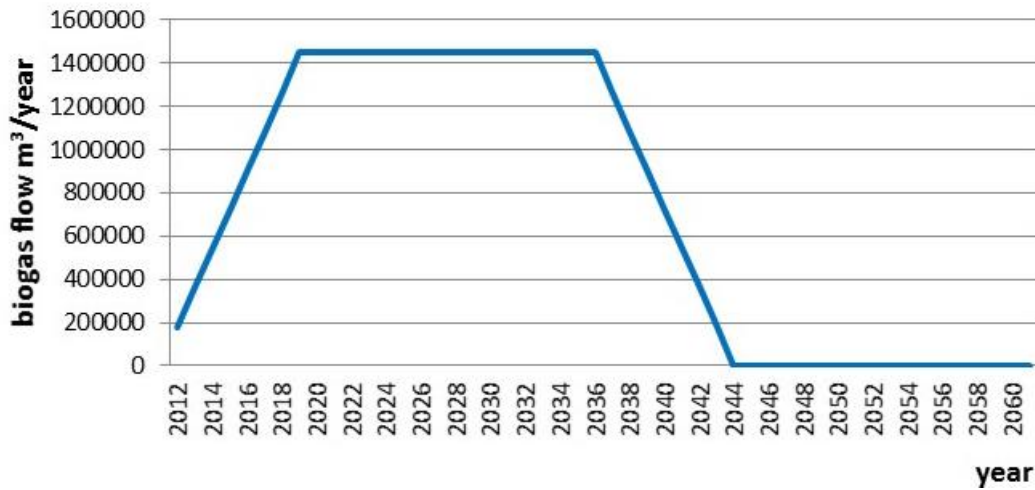
Figure 7. Biogas generation in the analyzed landfill
